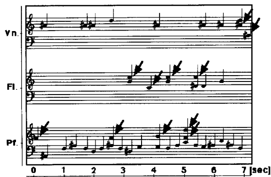
Fig. 10. Output of the system before introduction of music streams. Arrows show the incorrectly source-identified notes.
