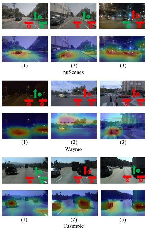
Fig. 6. There are SOB's predictions and explanations for 3 datasets. For each dataset, the first row is the prediction results, the second row is the corresponding explanations. We can see that not only the prediction results are correct but also the explanations. The SOB could make correct prediction results based on the right objects, such as vehicles; lanes, e.g., (2) in nuScenes, (1) in Waymo, (1) in Tusimple; pedestrians, e.g., (3) in Waymo; traffic light, e.g., (2) in Waymo.
